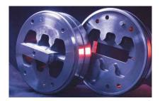
An extruding tool is completely processed within **a few minutes**. According to the processing time, surface values of Ra 0.2  $\mu$ m and Rz 1  $\mu$ m are obtained.
