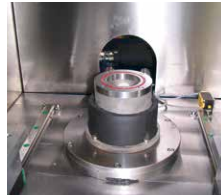
Within a short conversion time, you can reduce the diameter easily with the help of one or more reducing kits .
