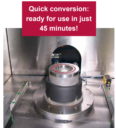
The diameter can be reduced quickly and easily in a short conversion time using one or more reducing kits.
